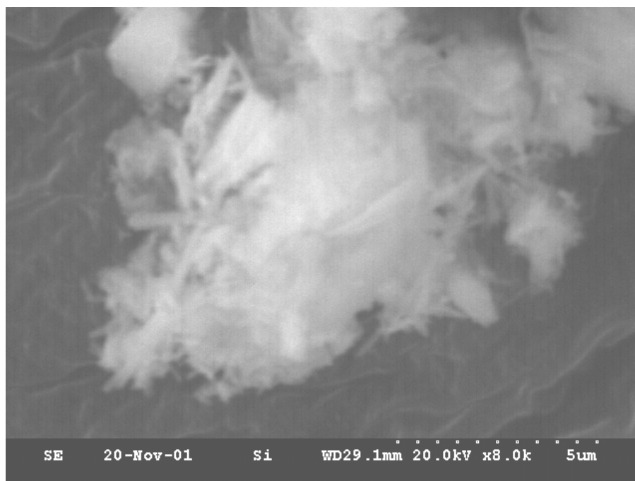
Figure 9.44. SEM image of ash from the eastern test boring in the ash platform at a depth of 50 to 52 feet. Long, thin particles are visible, and show evidence of cementitious phases forming.
